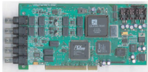
**Figure 19.** Time/frequency counter on a PC board with PCI interface.
